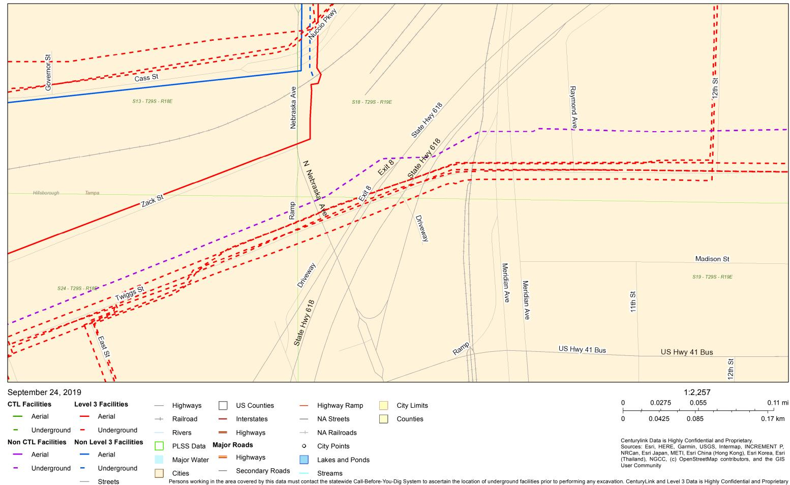
Persons working in the area covered by this data must contact the statewide Call-Before-You-Dig System to ascertain the location of underground facilities prior to performing any excavation. CenturyLink and Level 3 Data is Highly Confidential and Proprietary
